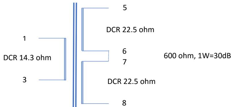
Figure 1. Wiring connections
